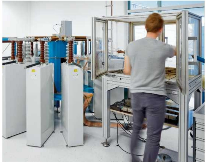
Fig. 27: Lightning surge current generator
